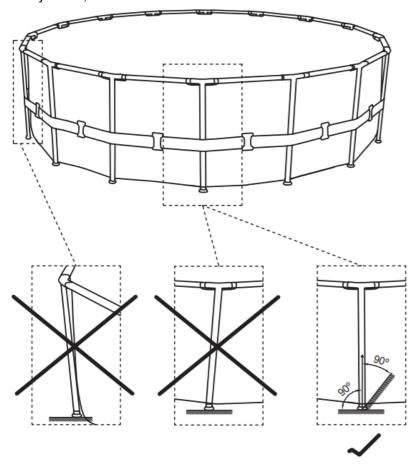
Do not assemble with pool legs on soft lawn. If you must assemble the pool on a soft surface, timber boards (not included) must be placed under the feet of the vertical support rods for even weight distribution. The timber board must meet two conditions:
